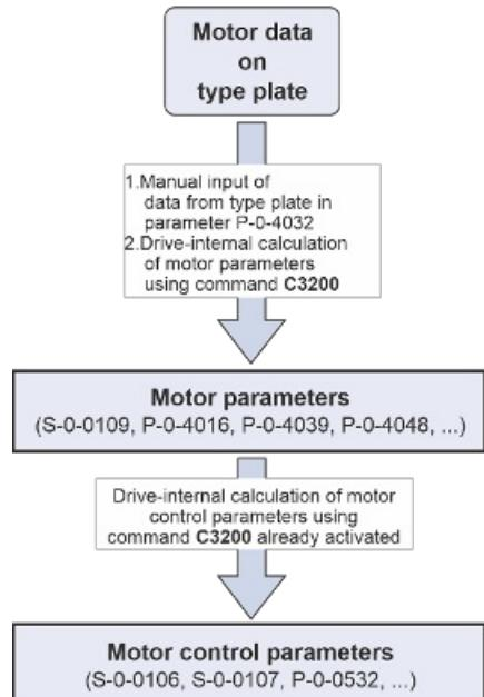
Fig. 306: Procedure and results of "C3200 Command Calculate motor data"
