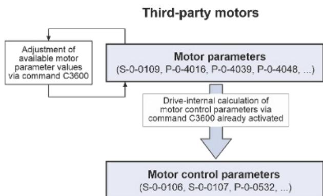
Fig. 307: Procedure and results of "C3600 Command Motor data identification"
