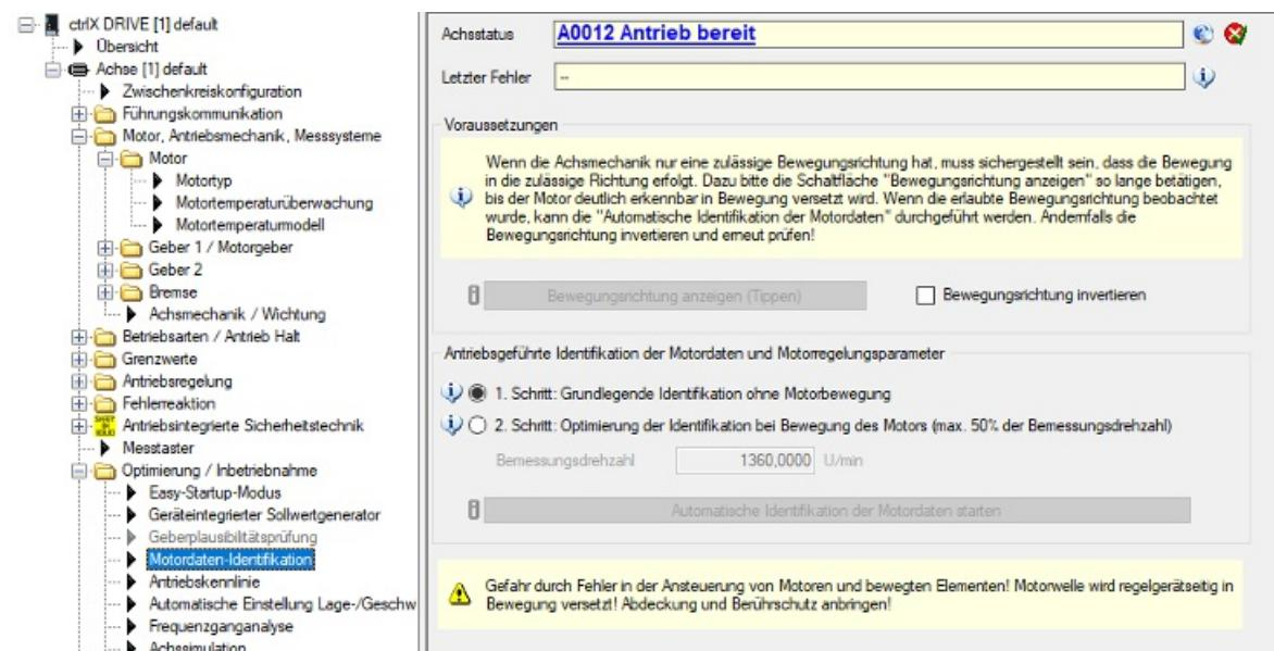
Fig. 304: ctrlX DRIVE Engineering dialog for motor data identification, selecting the drive-controlled identification, step 1
