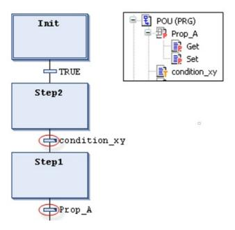
As opposed to CoDeSys V2.3, now PLC Engineering treats a transition condition like a method call. The entry has the following syntax:
